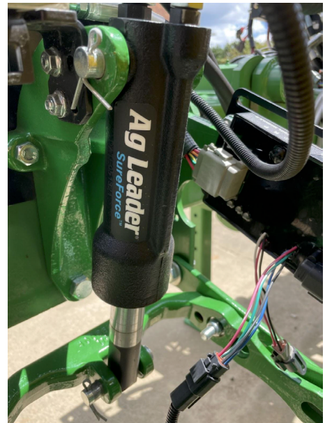
Figure 4. Hydraulic downforce may be increasingly important when planting at high speeds to ensure adequate seed depth. Image credit: Mike Mulvaney, Mississippi State University.
