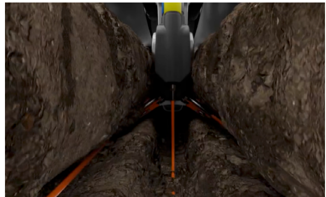
Figure 5. FurrowJet by Precision Planting places three streams of liquid fertilizer along the trench: One stream is with the seed, and two streams are in the sidewall. Image credit: https://www.precisionplanting.com/products/product/furrowjet .
